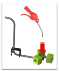
Once the filter is maintenance is completed, be sure to check all of the coolant and oil ports as well as the float tubes for obstructions. See above illustration
